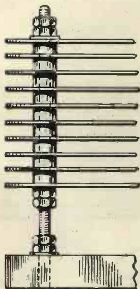
Fig. 2. Enlarged view showing the assembly of the fixed plates upon the side rods.
