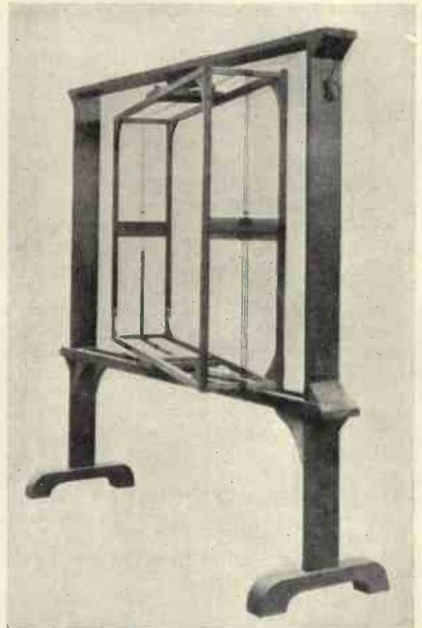
Fig. 11. A loop or frame aerial used for direction-finding purposes.
