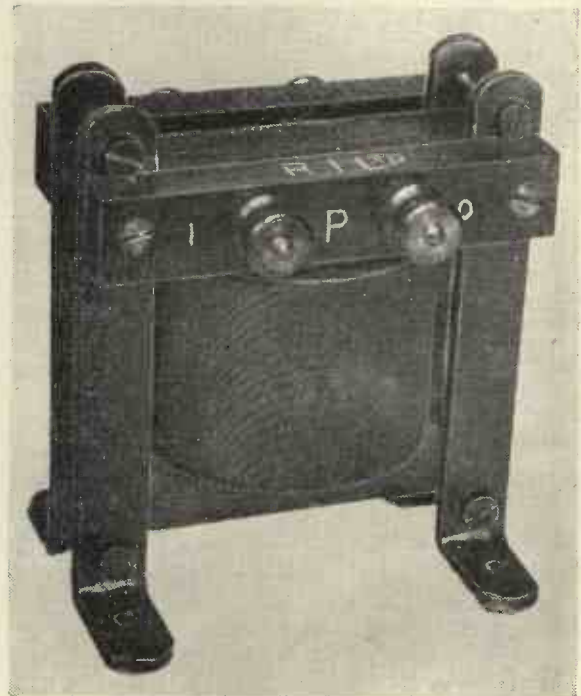
Fig. 7. L.F. transformer used in the sets described in this article.
