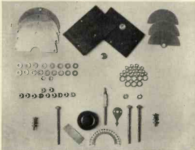
Complete set of parts for the assembly of a variable condenser of 0.0001 \mu F. capacity.
